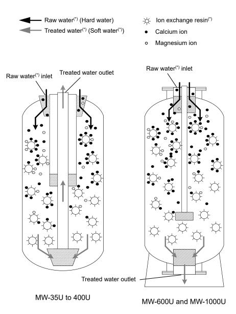
Figure 2-1: Mechanism of hardness(\*)-components removal
