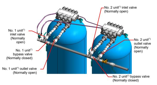
Figure 3-7: Locations of valves (MW-100U, 150U, MW-250U, and MW-400U)
