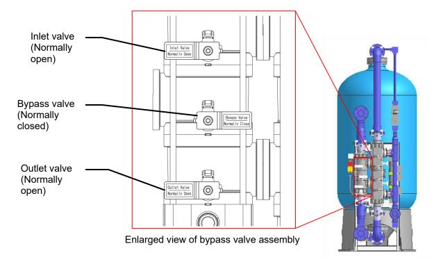
\* The state of the handles shown in the enlarged view above is the state during water flow<sup>(\*)</sup>.
