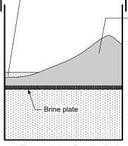
Make sure that there is enough regenerating salt<sup>(\*)</sup> in the tank to fill about 1/3 of the capacity of the tank at all times.
