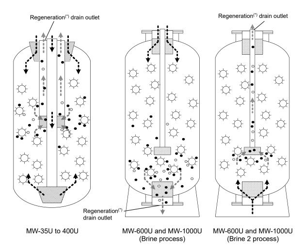
Figure 2-2: Regeneration mechanism of ion exchange resin(\*)
